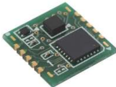
Figure 1.1.1: OMRON D7S Vibration Sensor
