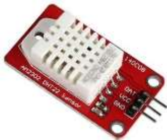
Figure 4.2.7: DHT22 Temperature and Humidity Sensor
