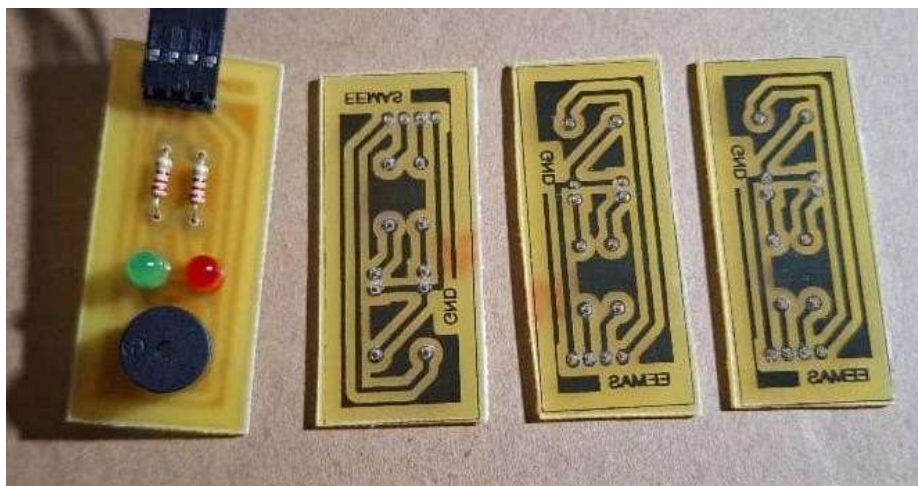
Figure 4.7.3: Assembled and Printed “EEMAS” Output Section PCB
